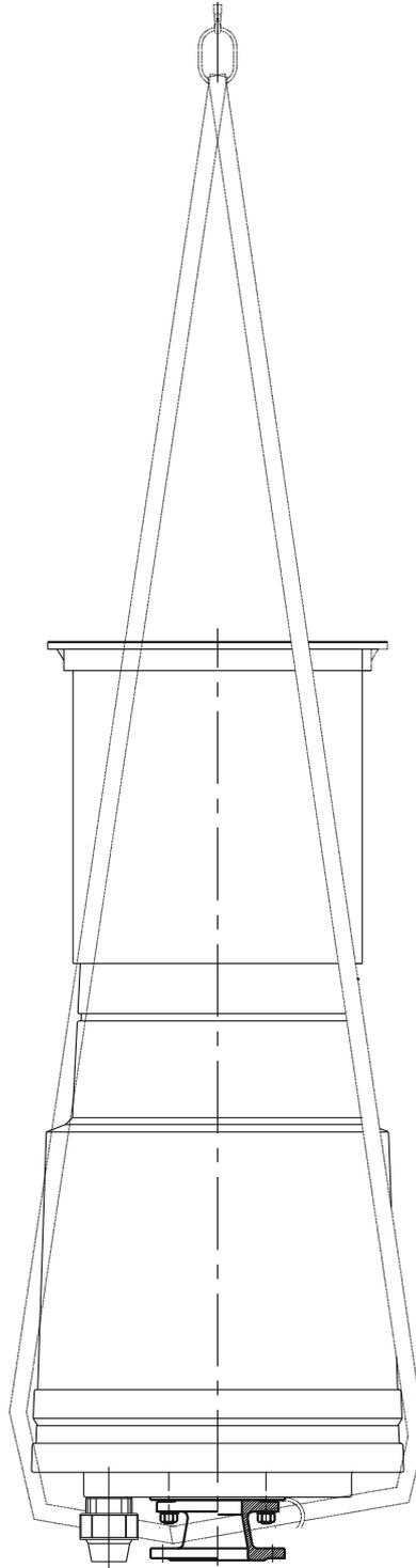
The manufacturer recommends slings for installation of the **TYPE 7090** valve.
