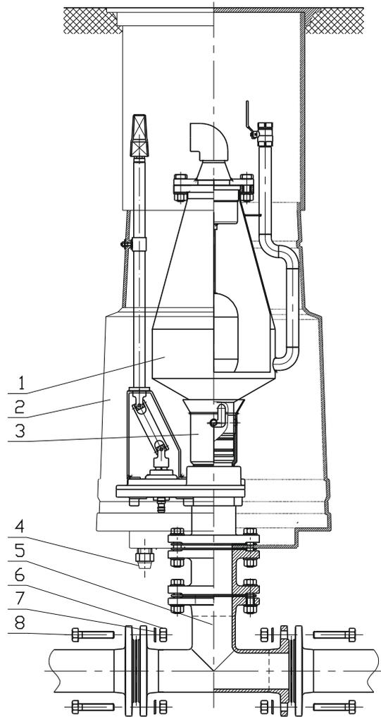
1. – Valve, type 7020 (or 7025); 2. – Well; 3. – QR coupling flange; 4. – Plastic connector; 5. – Tee; 6. – Nut; 7. – Washer; 8. – Bolt.
