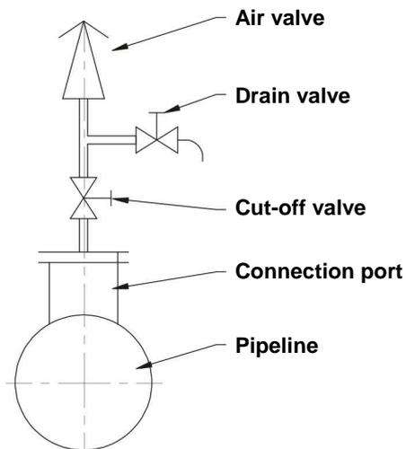
The connection port (turret) diameter must be adequately large and be at least the size of the air valve. The connection port orientation shall be vertical. The drain valve is intended for manual air relief or aeration, and for depressurizing (by draining) prior to maintenance work. The cut-off valve allows installing and removing the air valve and the drain valve.
