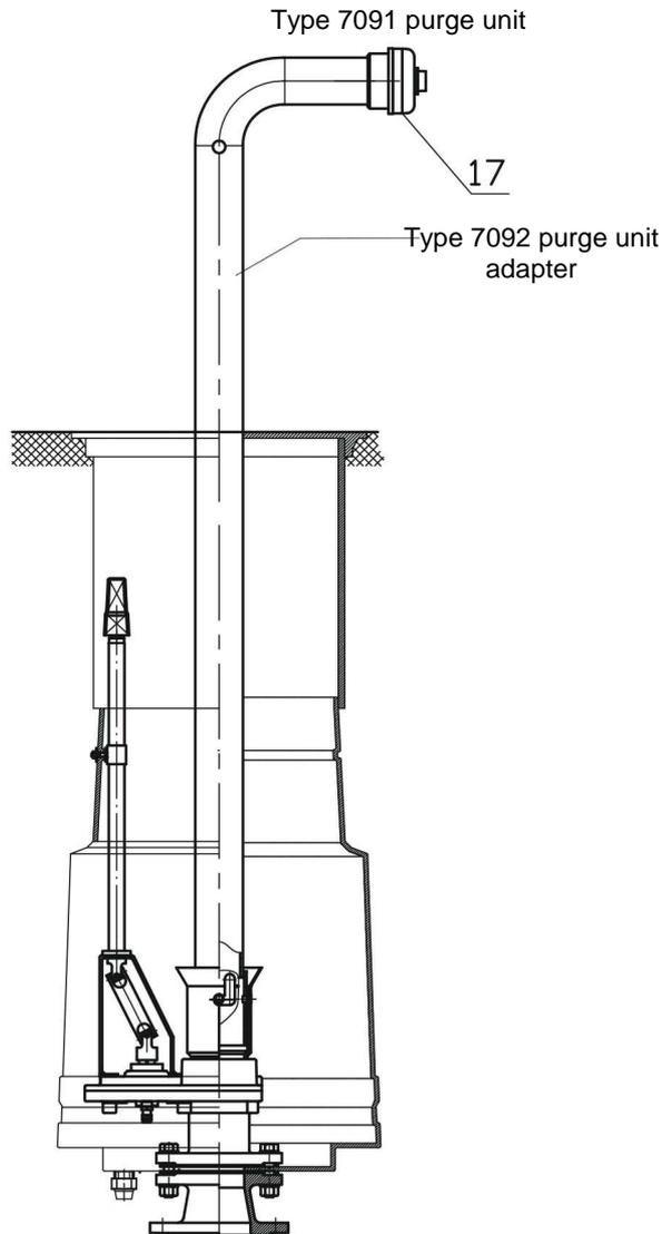
Using the purge unit: replace the Type 7020/7025 valve from the **TYPE 7090** air valve with the purge unit.
