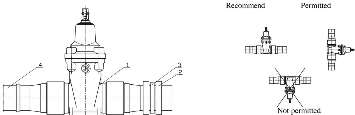
1. - Gate valve; 2. - Clamping parts; 3. - Heating element; 4. - PE 100 pipeline
